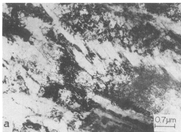
Fig. 7 Bright-field (a) and dark-field (b) micrographs showing internally twinned plates in the single-tempered steel
