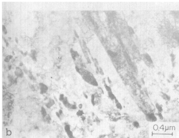
Fig. 4 Bright-field TEM micrographs of the single-tempered steel
